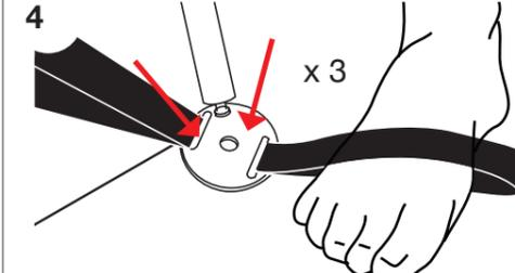
Insert one end of each pole into the eyelet of the base plate at the one end of the pole sleeve.
