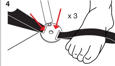
Insert one end of each pole into the eyelet of the base plate at the one end of the pole sleeve.
