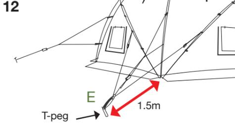
Stake out a long T-peg 1.5 m from each of the six corners and connect the guy lines.
