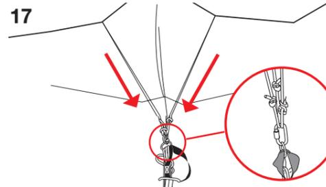
Connect the guy lines of the shade cover to the snap hooks on the T-pegs and tighten.
