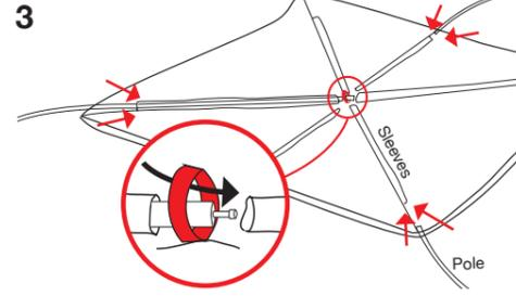
Slide three cross poles through the sleeves. Ensure that all poles go through the central red loop.
