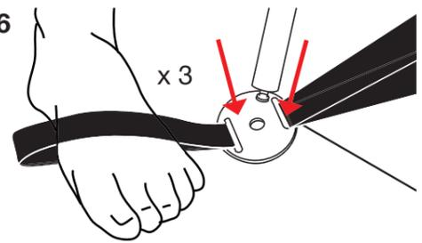
Insert the other end of each pole into the eyelet of the base plate at the other end of the pole sleeve.
