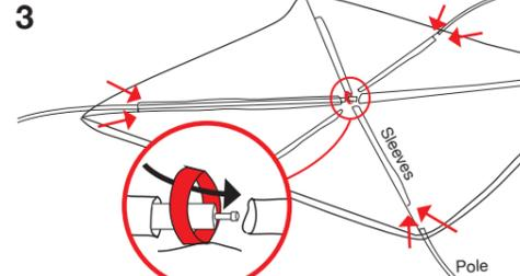
Slide three cross poles through the sleeves. Ensure that all poles go through the central red loop.
