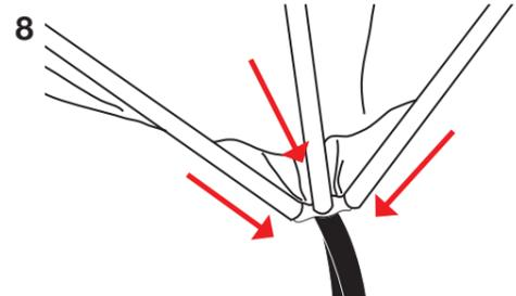
Fix the ends in the three-pole base plates at the sides of the tent.
