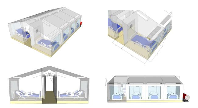
These modules are developed for triage, testing, isolation and treatment of patients infected by the Corona virus. Inspired by the LegendMEDI Ebola tent the cabins are made of easy to clean and disinfect PE or PVC coated polyester fabric with all seams heat welded to create easy to clean smooth surfaces.
