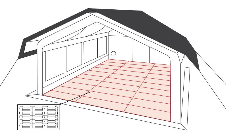
Modular flooring system for our multipurpose and MSU shelters. The pre-assembled tiles to allow for fast assembly on site and provide a non-slip surface for patients and staff. They are designed for easy cleaning and can be laid over cables.
