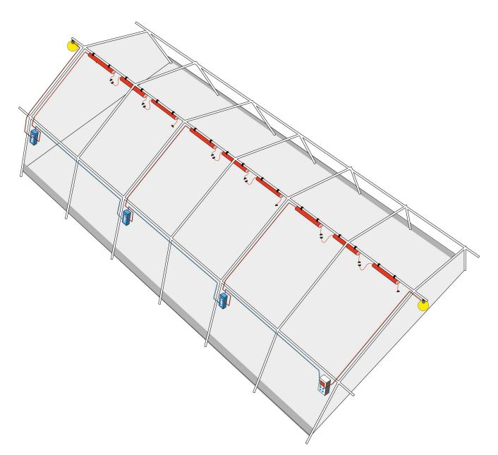
Each tent can be fit with an easily installed electrical lighting kit to provide tube lighting inside the tent, power sockets and also includes external lights above the doors. The light tubes can be individually turned on/off.
