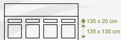
Side view (Window and ventilation)
