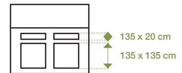
Side view (Window and ventilation)
