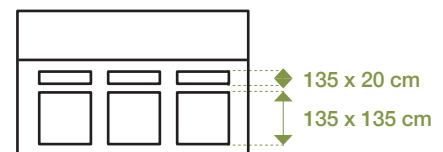
Side view (Window and ventilation)
