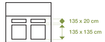
Side view (Window and ventilation)
