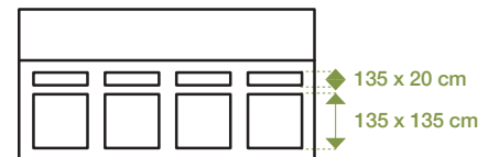
Side view (Window and ventilation)
