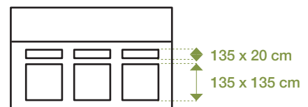
Side view (Window and ventilation)
