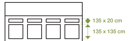
Side view (Window and ventilation)
