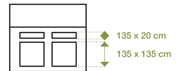
Side view (Window and ventilation)
