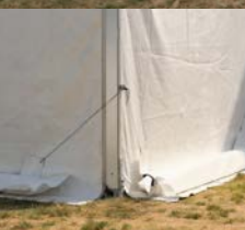
Ballast anchors (to be filled with sand, stones or water)
