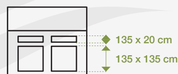
Side view (Window and ventilation)
