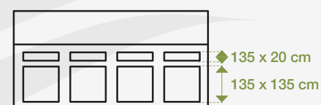
Side view (Window and ventilation)
