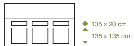
Side view (Window and ventilation)
