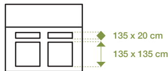
Side view (Window and ventilation)
