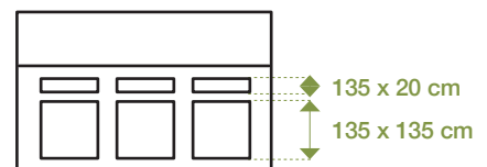
Side view (Window and ventilation)
