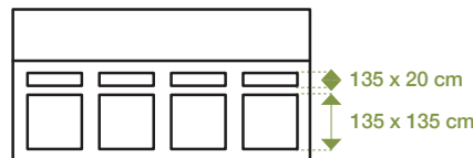
Side view (Window and ventilation)
