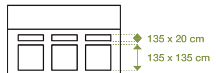
Side view (Window and ventilation)
